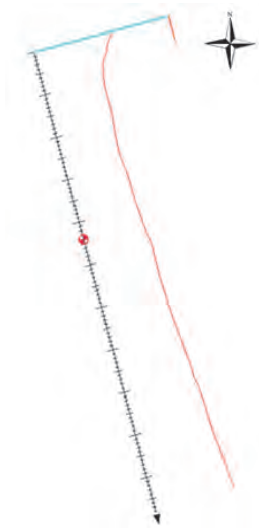
Figure 72. GenCade south domain, red line is the initial shoreline, blue and orange lines represent the composite south jetty.
